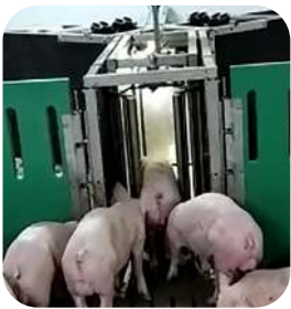
Cage weighed and arch of entry to limit access
